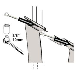
C With 3/8 in (10mm) socket wrench, loosely screw two 1/4 inch x 3 inch Lag Bolts with flat washers C through top Wall Mount slots into stud or plywood backing. Hint: Coat all bolts' threads with beeswax, paraffin, candle wax or soap for easy & safe wrenching.
