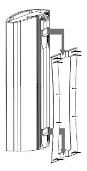
B Using a mechanical lift or enough manpower to be safe, move the speaker to the Wall Mount; lift the speaker with the Spine's two male ends above and over the Wall Mount's female hangers. Slowly lower them on to the hangers, ensuring that both top & bottom are securely hung.
