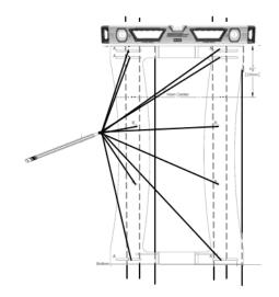
Using Wall Mount Template B, determine speaker location on the wall. Slots MUST be backed by studs or wood. Note that the speaker's acoustic center (tweeter vertical mid point) is 10-1/2 inches (267mm) below the top of the wall mount.. Level or align. Mark all 10 slots & holes with pencil.
