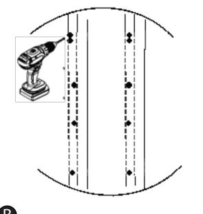
With 7/32 inch 5.5 mm (preferred) or 3/16 inch 5mm bit, drill pilot holes through wall surface into studs or wood backing through your marked holes. If any of the 4 center holes are not over studs or wood backing, install included anchors. For safety, use all 10 holes.
