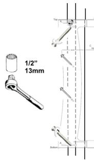
D Screw 4 Lag bolts & washers through remaining 4 slots. Minimum 6 lag bolts MUST be used. Test for sheer strength. To keep Wall Mount from vibrating, you must screw remaining 4 holes with the #10 X 1.25" oval screws and anchors (if needed) or other fasteners appropriate for your wall type.
